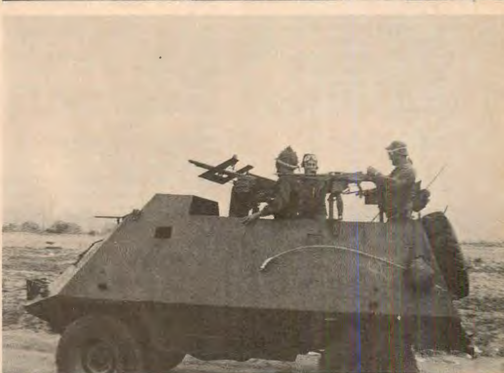
TOP: Panhard armored car carrying 90mm gun is mainstay of ZR Armor Corps. Recently, ZR forces captured and returned to ZR an unspecified number of Russian T-54 tanks from Mozambique. BOTTOM: Rhodesian "home grown" armored scout vehicle, carries twin Browning light MG's in front and MAG light MG on side. For more information on twin Brownings and Rhodesian-developed armor, see January 1979, SOF.
